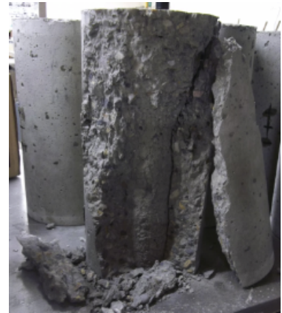
Photo depicting ruptured cylinder
